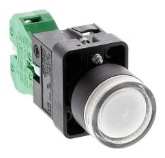
AutomationDirect pushbutton, IP65, 22mm, momentary, incandescent illuminated, (1) N.O. contact(s), plastic base, plastic bezel, plastic ring, Operator: clear, flush, 30mm, round, plastic, 24 VAC/VDC, full voltage.
