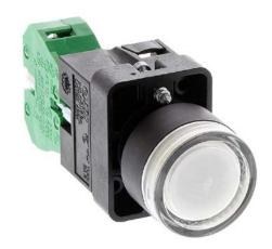
AutomationDirect pushbutton, IP65, 22mm, momentary, incandescent illuminated, (1) N.O. contact(s), plastic base, plastic bezel, plastic ring, Operator: clear, flush, 30mm, round, plastic, 24 VAC/VDC, full voltage.
