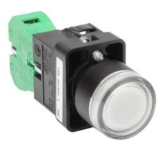
AutomationDirect pushbutton, IP65, 22mm, momentary, LED illuminated, (1) N.O. contact(s), plastic base, plastic bezel, plastic ring, Operator: clear, flush, 30mm, round, plastic, 120 VAC/VDC, full voltage.
