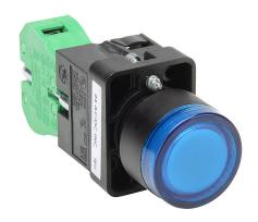
AutomationDirect pushbutton, IP65, 22mm, momentary, incandescent illuminated, (1) N.O. contact(s), plastic base, plastic bezel, plastic ring, Operator: blue, flush, 30mm, round, plastic, 24 VAC/VDC, full voltage.
