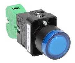
AutomationDirect pushbutton, IP65, 22mm, momentary, LED illuminated, (1) N.O. contact(s), plastic base, plastic bezel, plastic ring, Operator: blue, flush, 30mm, round, plastic, 24 VAC/VDC, full voltage.
