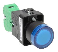
AutomationDirect pushbutton, IP65, 22mm, momentary, incandescent illuminated, (1) N.O. contact(s), plastic base, plastic bezel, plastic ring, Operator: blue, flush, 30mm, round, plastic, 120 VAC/VDC, full voltage.
