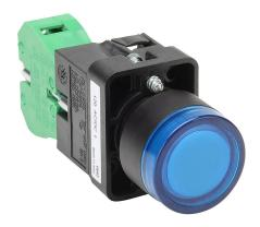
AutomationDirect pushbutton, IP65, 22mm, momentary, LED illuminated, (1) N.O. contact(s), plastic base, plastic bezel, plastic ring, Operator: blue, flush, 30mm, round, plastic, 120 VAC/VDC, full voltage.
