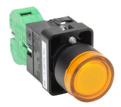
AutomationDirect pushbutton, IP65, 22mm, momentary, LED illuminated, (1) N.O. contact(s), plastic base, plastic bezel, plastic ring, Operator: yellow, flush, 30mm, round, plastic, 120 VAC/VDC, full voltage.
