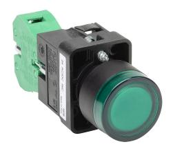
AutomationDirect pushbutton, IP65, 22mm, momentary, incandescent illuminated, (1) N.O. contact(s), plastic base, plastic bezel, plastic ring, Operator: green, flush, 30mm, round, plastic, 24 VAC/VDC, full voltage.
