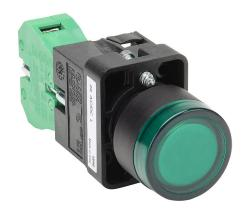
AutomationDirect pushbutton, IP65, 22mm, momentary, LED illuminated, (1) N.O. contact(s), plastic base, plastic bezel, plastic ring, Operator: green, flush, 30mm, round, plastic, 24 VAC/VDC, full voltage.
