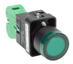
AutomationDirect pushbutton, IP65, 22mm, momentary, LED illuminated, (1) N.O. contact(s), plastic base, plastic bezel, plastic ring, Operator: green, flush, 30mm, round, plastic, 120 VAC/VDC, full voltage.
