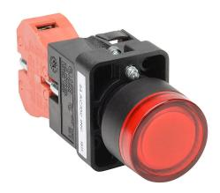
AutomationDirect pushbutton, IP65, 22mm, momentary, incandescent illuminated, (1) N.C. contact(s), plastic base, plastic bezel, plastic ring, Operator: red, flush, 30mm, round, plastic, 24 VAC/VDC, full voltage.
