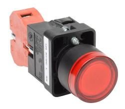
AutomationDirect pushbutton, IP65, 22mm, momentary, LED illuminated, (1) N.C. contact(s), plastic base, plastic bezel, plastic ring, Operator: red, flush, 30mm, round, plastic, 120 VAC/VDC, full voltage.
