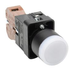
AutomationDirect pushbutton, IP65, 22mm, push ON - push OFF, LED illuminated, (1) N.O. contact(s), plastic base, plastic bezel, plastic ring, Operator: white, flush, 30mm, round, plastic, 24 VAC/ VDC, full voltage.
