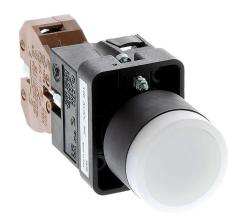
AutomationDirect pushbutton, IP65, 22mm, push ON - push OFF, incandescent illuminated, (1) N.O. contact(s), plastic base, plastic bezel, plastic ring, Operator: white, flush, 30mm, round, plastic, 120 VAC/VDC, full voltage.
