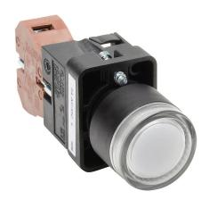
AutomationDirect pushbutton, IP65, 22mm, push ON - push OFF, LED illuminated, (1) N.O. contact(s), plastic base, plastic bezel, plastic ring, Operator: clear, flush, 30mm, round, plastic, 24 VAC/VDC, full voltage.
