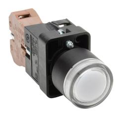
AutomationDirect pushbutton, IP65, 22mm, push ON - push OFF, incandescent illuminated, (1) N.O. contact(s), plastic base, plastic bezel, plastic ring, Operator: clear, flush, 30mm, round, plastic, 120 VAC/VDC, full voltage.
