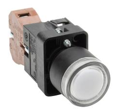
AutomationDirect pushbutton, IP65, 22mm, push ON - push OFF, LED illuminated, (1) N.O. contact(s), plastic base, plastic bezel, plastic ring, Operator: clear, flush, 30mm, round, plastic, 120 VAC/VDC, full voltage.
