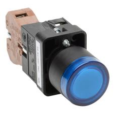
AutomationDirect pushbutton, IP65, 22mm, push ON - push OFF, incandescent illuminated, (1) N.O. contact(s), plastic base, plastic bezel, plastic ring, Operator: blue, flush, 30mm, round, plastic, 24 VAC/VDC, full voltage.
