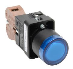
AutomationDirect pushbutton, IP65, 22mm, push ON - push OFF, LED illuminated, (1) N.O. contact(s), plastic base, plastic bezel, plastic ring, Operator: blue, flush, 30mm, round, plastic, 24 VAC/VDC, full voltage.
