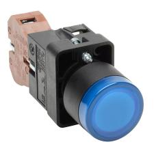
AutomationDirect pushbutton, IP65, 22mm, push ON - push OFF, incandescent illuminated, (1) N.O. contact(s), plastic base, plastic bezel, plastic ring, Operator: blue, flush, 30mm, round, plastic, 120 VAC/VDC, full voltage.
