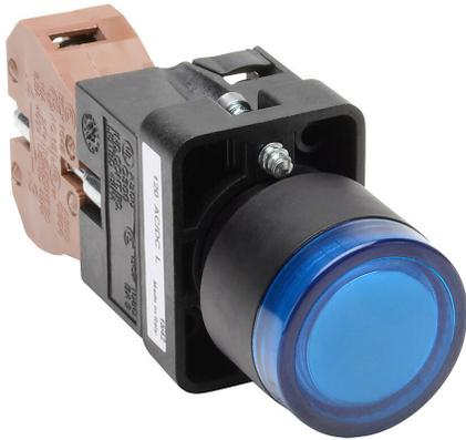
AutomationDirect pushbutton, IP65, 22mm, push ON - push OFF, LED illuminated, (1) N.O. contact(s), plastic base, plastic bezel, plastic ring, Operator: blue, flush, 30mm, round, plastic, 120 VAC/VDC, full voltage.
