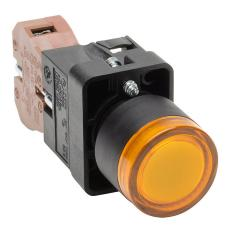
AutomationDirect pushbutton, IP65, 22mm, push ON - push OFF, LED illuminated, (1) N.O. contact(s), plastic base, plastic bezel, plastic ring, Operator: yellow, flush, 30mm, round, plastic, 24 VAC/ VDC, full voltage.
