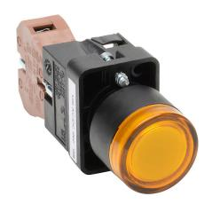
AutomationDirect pushbutton, IP65, 22mm, push ON - push OFF, incandescent illuminated, (1) N.O. contact(s), plastic base, plastic bezel, plastic ring, Operator: yellow, flush, 30mm, round, plastic, 120 VAC/VDC, full voltage.
