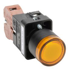
AutomationDirect pushbutton, IP65, 22mm, push ON - push OFF, LED illuminated, (1) N.O. contact(s), plastic base, plastic bezel, plastic ring, Operator: yellow, flush, 30mm, round, plastic, 120 VAC/VDC, full voltage.
