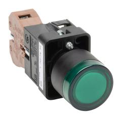
AutomationDirect pushbutton, IP65, 22mm, push ON - push OFF, LED illuminated, (1) N.O. contact(s), plastic base, plastic bezel, plastic ring, Operator: green, flush, 30mm, round, plastic, 24 VAC/ VDC, full voltage.
