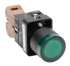
AutomationDirect pushbutton, IP65, 22mm, push ON - push OFF, incandescent illuminated, (1) N.O. contact(s), plastic base, plastic bezel, plastic ring, Operator: green, flush, 30mm, round, plastic, 120 VAC/VDC, full voltage.
