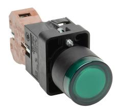
AutomationDirect pushbutton, IP65, 22mm, push ON - push OFF, LED illuminated, (1) N.O. contact(s), plastic base, plastic bezel, plastic ring, Operator: green, flush, 30mm, round, plastic, 120 VAC/VDC, full voltage.
