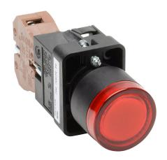
AutomationDirect pushbutton, IP65, 22mm, push ON - push OFF, incandescent illuminated, (1) N.O. contact(s), plastic base, plastic bezel, plastic ring, Operator: red, flush, 30mm, round, plastic, 24 VAC/VDC, full voltage.
