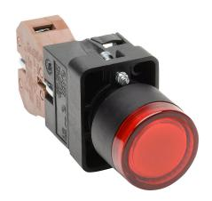
AutomationDirect pushbutton, IP65, 22mm, push ON - push OFF, LED illuminated, (1) N.O. contact(s), plastic base, plastic bezel, plastic ring, Operator: red, flush, 30mm, round, plastic, 24 VAC/VDC, full voltage.
