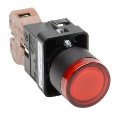
AutomationDirect pushbutton, IP65, 22mm, push ON - push OFF, incandescent illuminated, (1) N.O. contact(s), plastic base, plastic bezel, plastic ring, Operator: red, flush, 30mm, round, plastic, 120 VAC/VDC, full voltage.
