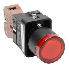
AutomationDirect pushbutton, IP65, 22mm, push ON - push OFF, LED illuminated, (1) N.O. contact(s), plastic base, plastic bezel, plastic ring, Operator: red, flush, 30mm, round, plastic, 120 VAC/VDC, full voltage.
