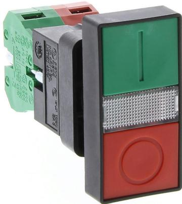
AutomationDirect pushbutton, IP40, 22mm, momentary, incandescent illuminated, (1) N.O./ (1) N.C. contact(s), plastic base, plastic bezel, Operator: red/green, double headed, 50mm, rectangular, plastic, operator text "(I) and (O)", 24 VAC/VDC, full voltage.
