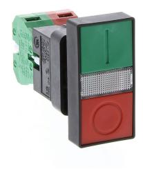
AutomationDirect pushbutton, IP40, 22mm, momentary, incandescent illuminated, (1) N.O./(1) N.C. contact(s), plastic base, plastic bezel, Operator: red/green, double headed, 50mm, rectangular, plastic, operator text "(I) and (0)", 24 VAC/VDC, full voltage.
