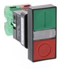
AutomationDirect pushbutton, IP40, 22mm, momentary, incandescent illuminated, (1) N.O./(1) N.C. contact(s), plastic base, plastic bezel, Operator: red/green, double headed, 50mm, rectangular, plastic, operator text "(I) and (0)", 120 VAC/VDC, full voltage.
