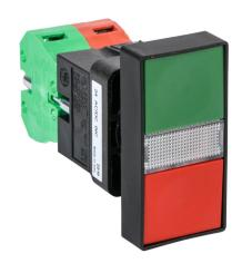
AutomationDirect pushbutton, IP40, 22mm, momentary, incandescent illuminated, (1) N.O./(1) N.C. contact(s), plastic base, plastic bezel, Operator: red/green, double headed, 60mm, rectangular, plastic, 24 VAC/VDC, full voltage.
