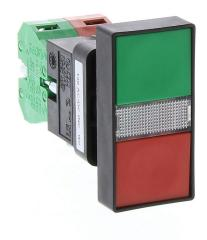
AutomationDirect pushbutton, IP40, 22mm, momentary, incandescent illuminated, (1) N.O./(1) N.C. contact(s), plastic base, plastic bezel, Operator: red/green, double headed, 60mm, rectangular, plastic, 120 VAC/VDC, full voltage.
