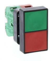
AutomationDirect pushbutton, IP65, 22mm, momentary, (1) N.O./ (1) N.C. contact(s), plastic base, plastic bezel, Operator: red/green, double headed, 60mm, rectangular, plastic.
