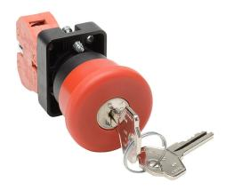
AutomationDirect emergency stop pushbutton, IP65, 22mm, key operated release, (1) N.C. contact(s), plastic base, plastic bezel, Operator: red, mushroom, 40mm, round, plastic.
