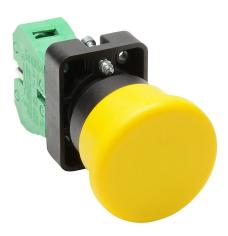
AutomationDirect pushbutton, IP65, 22mm, momentary, (1) N.O. contact(s), plastic base, plastic bezel, Operator: yellow, mushroom, 40mm, round, plastic.
