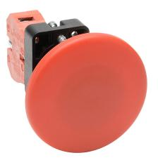
AutomationDirect pushbutton, IP65, 22mm, momentary, (1) N.C. contact(s), plastic base, plastic bezel, Operator: red, mushroom, 60mm, round, plastic.
