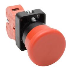
AutomationDirect pushbutton, IP65, 22mm, momentary, (1) N.C. contact(s), plastic base, plastic bezel, Operator: red, mushroom, 40mm, round, plastic.
