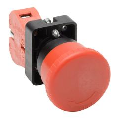
AutomationDirect emergency stop pushbutton, IP65, 22mm, twist-to-release, (1) N.C. contact(s), plastic base, plastic bezel, Operator: red, mushroom, 40mm, round, plastic.
