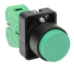
AutomationDirect pushbutton, IP65, 22mm, momentary, (1) N.O. contact(s), plastic base, plastic bezel, Operator: green, extended, 30mm, round, plastic.
