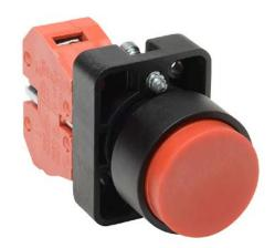
AutomationDirect pushbutton, IP65, 22mm, momentary, (1) N.C. contact(s), plastic base, plastic bezel, Operator: red, extended, 30mm, round, plastic.
