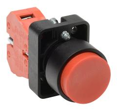
AutomationDirect pushbutton, IP65, 22mm, momentary, (1) N.C. contact(s), plastic base, plastic bezel, Operator: red, extended, 30mm, round, plastic.
