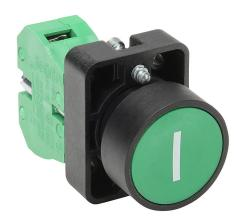
AutomationDirect pushbutton, IP65, 22mm, momentary, (1) N.O. contact(s), plastic base, plastic bezel, Operator: green, flush, 30mm, round, plastic, operator text "(I)".
