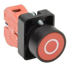
AutomationDirect pushbutton, IP65, 22mm, momentary, (1) N.C. contact(s), plastic base, plastic bezel, Operator: red, flush, 30mm, round, plastic, operator text "(O)".
