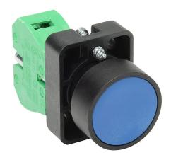
AutomationDirect pushbutton, IP65, 22mm, momentary, (1) N.O. contact(s), plastic base, plastic bezel, Operator: blue, flush, 30mm, round, plastic.
