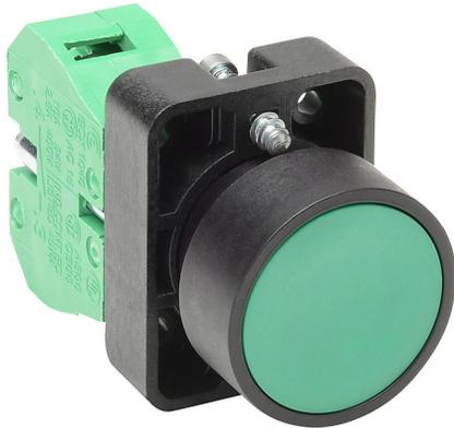
AutomationDirect pushbutton, IP65, 22mm, momentary, (1) N.O. contact(s), plastic base, plastic bezel, Operator: green, flush, 30mm, round, plastic.
