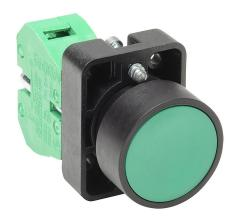
AutomationDirect pushbutton, IP65, 22mm, momentary, (1) N.O. contact(s), plastic base, plastic bezel, Operator: green, flush, 30mm, round, plastic.
