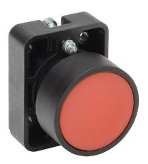
AutomationDirect pushbutton, IP65, 22mm, momentary, operator only, plastic base, plastic bezel, Operator: red, flush, 30mm, round, plastic.
