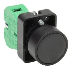
AutomationDirect pushbutton, IP65, 22mm, momentary, (1) N.O. contact(s), plastic base, plastic bezel, Operator: black, flush, 30mm, round, plastic.
