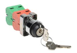
AutomationDirect selector switch, 22mm, 3-position, maintained, key removable in all positions, (2) N.O./(2) N.C. contact(s), metal base, metal bezel, Operator: black, key, 30mm, round, plastic.
